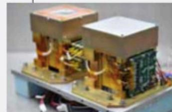
X-ray sensor and signal-processing electronics
