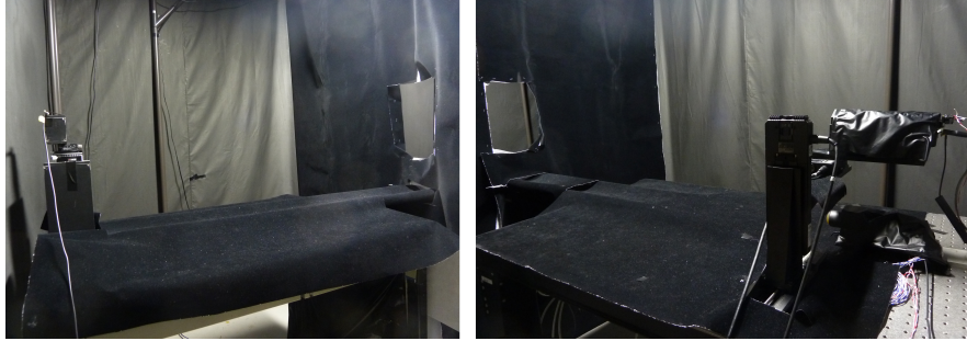
FIGURE 3.18: The performance evaluation system in real. Left: left side of dark room with LED at the leftmost. Right: right side of dark room with PMT and light concentrator at the rightmost.
