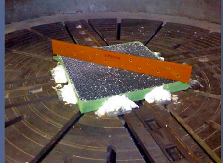
Mold R=55.2m after machining
